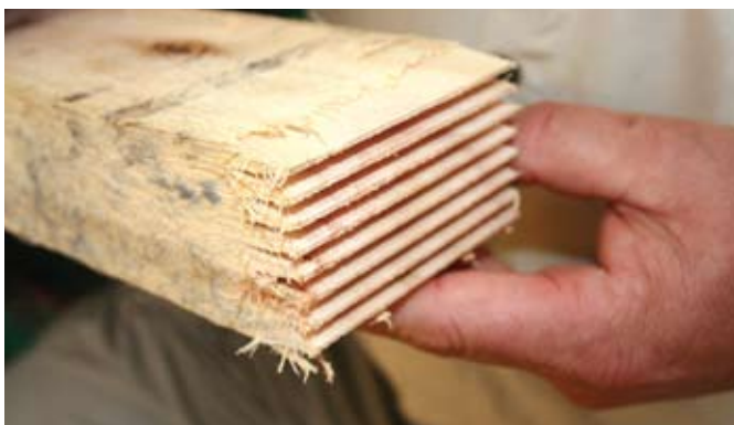
The fingerjoint made on the profiler
