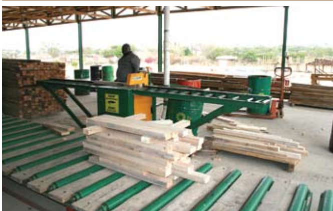
The start of the Biligom® production line where defects are cross-cut from the planks
